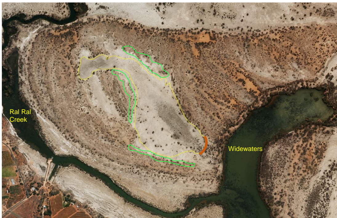
Figure 11: Widewaters West environmental watering site. The yellow polygon indicates the extent of inundation during a 'standard' environmental watering event. The green polygons represent areas which contain black box recruits from the 2010-12 floods. The brown bar represents a proposed retention bank.
