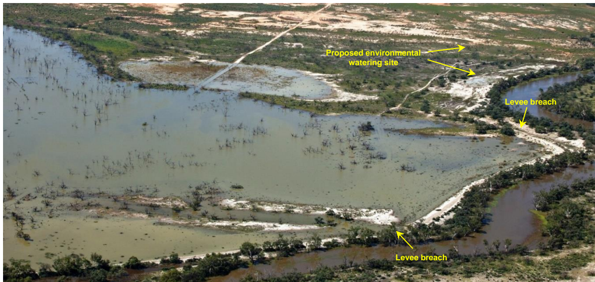
Figure 9: The southern Woolpolool floodplain in March 2011 showing the lack of connectivity between the floodplain and Ral Ral creek (right of picture) due to the Ral Ral levee.
